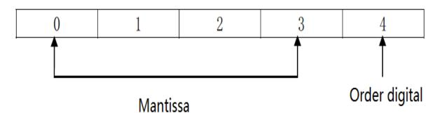
Definition of floating point numbers using scientific notation, decimal point after the first BCD code, the composition structure of 5 bytes, the first four bytes mantissa, after a byte-order code, order code MSB number symbol, for the second high-order character ("0" represents a positive number, "1" represents a negative number), for the six low-order code value in the range of 0-63H
